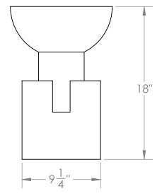
Made of cold rolled steel, the table is finished in a light antique brass with a dark antique brass block base. The contrasting finishes accentuate the interlocking shapes.
