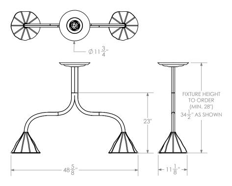
Sinuous curves of carved hardwood terminate in hand-upholstered conical silk shades, with a classically inspired wood ceiling rose. Inside each shade, a hand blown white glass teardrop houses the light source.
