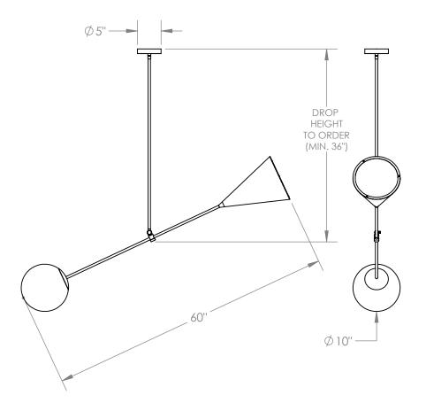
A conical light source at one end and a handblown matte white glass orb on the other hold this piece in balance. The central hinge mechanism allows adjustment of the fixture to any desired angle.
