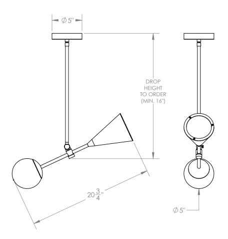
A conical light source at one end and a handblown matte white glass orb on the other hold this piece in balance. The central hinge mechanism allows adjustment of the fixture to any desired angle.
